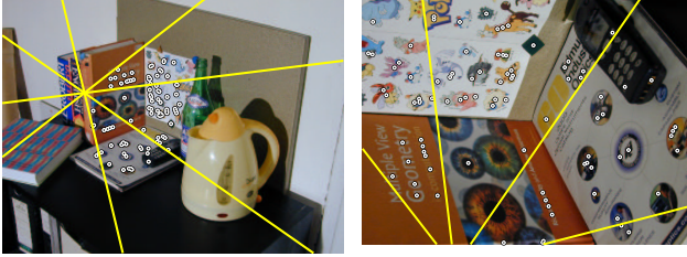
Fig. 7: Epipolar lines and 84 detected correspondences (markers) superimposed over the ‘Bookshelf’ pair.
