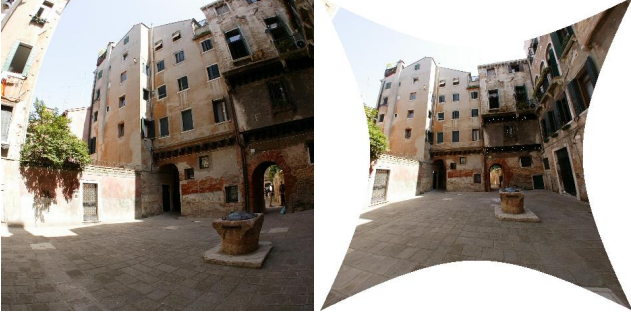
Fig. 4: ‘Courtyard QY’ image pair, 48% of inliers. High radial distortion example. Central part (1400 x 1400 pixels, view field 100°) of the fish-eye images. Original first image on the left, second (different) image with RD removed on right.
