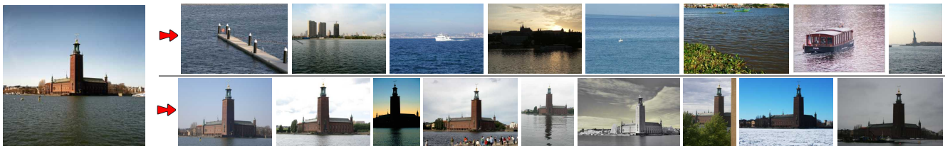
Figure 1. A query image (left) and top ranked images retrieved by two methods from a database of 5 million images: standard ( tf-idf with spatial verification) retrieval (top) and the same method after automatic detection and removal of co-ocset features (bottom).
