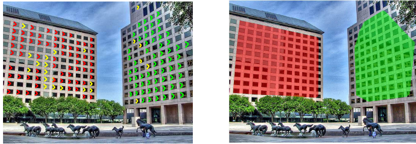
Fig. 7. Two planar surfaces with a repetitive pattern segmented by RANSAC. Left: one group of matching features, inliers to one model in red, the other in green, outliers to both models in yellow. Right: the convex hull of consistent features.
