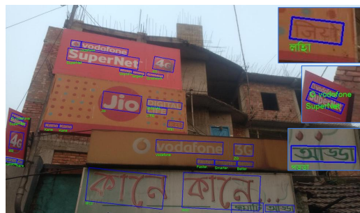
Figure 1: Text in multiple languages appearing in a scene. The proposed E2E-MLT method localizes words, predicts the scripts and generates a text transcription for each bounding box.
