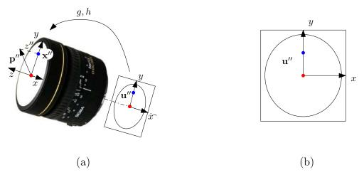
Figure 3.2: Omnidirectional image formation: (a) Projection of a scene point to a sensor plane. (b) The sensor plane with field of view circle. (Adopted from [6])
