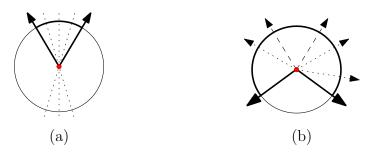
Figure 3.1: (a) Directional camera. Scene points are represented by straight lines. (b) Omnidirectional camera. Scene points are represented by half-lines. (Adopted from [6])
