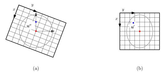
Figure 3.3: Omnidirectional image formation: (a, b) Digitization process – affine transformation of the field of view circle. (Adopted from [6])
