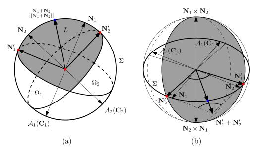
Figure 5.6: The epipolar alignment of  $\Omega_i$ , i = 1, 2 with the assumption that the visible angle of both cameras is 180°. Both figure (a) and (b) depict the identical situation, only from a different viewpoints
