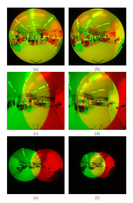
Figure B.14: (a) Overlay of  $P_{O_1}, \mathcal{P}_{O_1}^1$  in the red channel,  $\mathcal{P}_{O_1}^2$  in the green channel. (b) Overlay of  $P_{O_2}, \mathcal{P}_{O_2}^1$  in the red channel,  $\mathcal{P}_{O_2}^2$  in the green channel. (c,d) Overlay of stereographic rectification of  $P_{O_1}$  and  $P_{O_2}$  respectively, param = 1. (e,f) Overlay of stereographic rectification of  $P_{O_1}$  and  $P_{O_2}$  respectively, param = 2.7.
