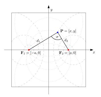
Figure 5.2: Bipolar coordinate system. A few  $\sigma$  isosurfaces are shown as dotted circles, dashed circles denote  $\tau$  isosurfaces .
