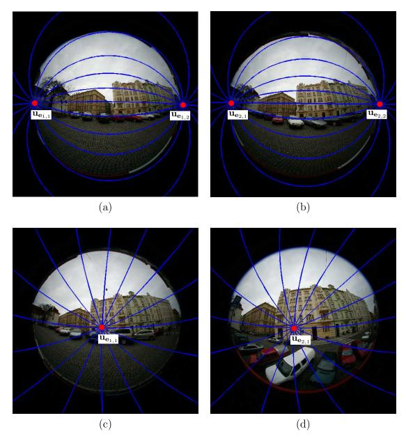
Figure B.1: (a, b) The image pair  $P_L = [\mathcal{P}_L^1, \mathcal{P}_L^2]$  acquired by a lateral motion of the camera. (b, c) The image pair  $P_F = [\mathcal{P}_F^1, \mathcal{P}_F^2]$  acquired by a forward motion of the camera.
