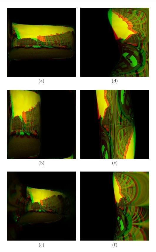
Figure B.7: (a, b, c) Overlay of spherical, swapped spherical and bipolar rectification of  $P_L$  respectively. (d, e, f) Overlay of spherical, swapped spherical and bipolar rectification of  $P_F$  respectively.
