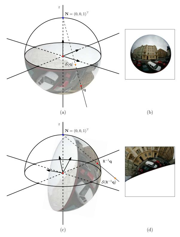
Figure 5.5: The effect of the change of the center of stereographic projection on a calibrated omnidirectional image. (a) The unit sphere colored using calibration transformation. (b) Stereographic projection of the calibrated image. (c) The unit sphere transformed by an arbitrary orthogonal matrix  $\mathbb{R}^{-1}$ . (d) Stereographic projection of the transformed sphere.
