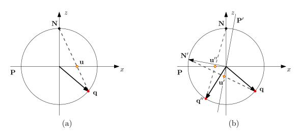
Figure 4.1: Stereographic projection: (a) Projection of a vector  $\mathbf{q} \in \mathbb{S}^3$  onto a vector  $\mathbf{u} \in \mathbb{R}^2$  by means of central projection from the North Pole N to the plane P. (b) Projection of a vector  $\mathbf{q} \in \mathbb{S}^3$  from N' to the plane P' is equivalent to the projection of a vector  $\mathbf{q}''$  to a vector  $\mathbf{u}''$  under the canonical stereographic projection, i.e.,  $\mathbf{u}'_{\mathbf{p}'} = \mathbf{u}''_{\mathbf{p}}$ .
