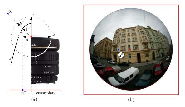
Figure 3.4: Mapping of a scene point **X** into a sensor plane point  $\mathbf{u}''$  for a fish-eye lens. Since orthographic camera projection is assumed, h = 1. (Adopted from [6])
