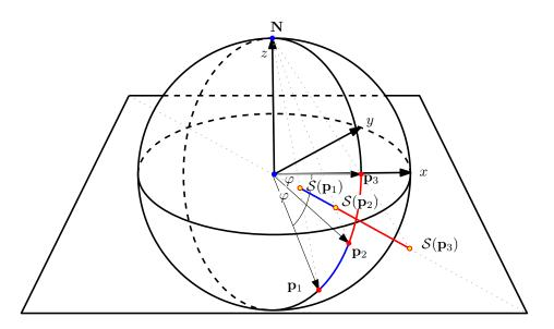
Figure 5.4: Spherically equidistantly positioned vectors  $\mathbf{p}_1, \mathbf{p}_2, \mathbf{p}_3$  and their respective stereographic transformations  $\mathcal{S}(\mathbf{p}_1), \mathcal{S}(\mathbf{p}_2), \mathcal{S}(\mathbf{p}_3)$ .
