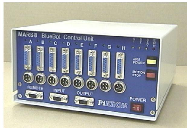
Dimensions of complete boxed system are 240 mm x 120 mm x 300 mm.
