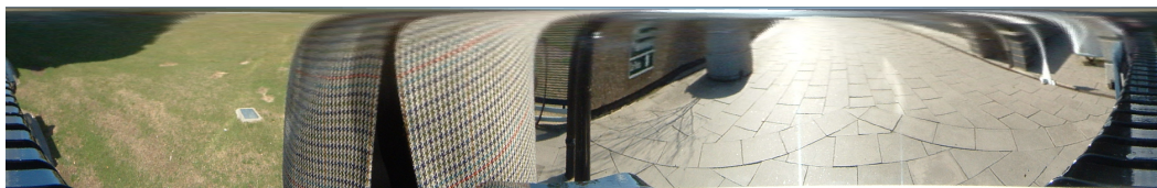
Fig. 7. Unwarping of Figure 2 showing the correct linear perspective of the straight edges on the paving.
