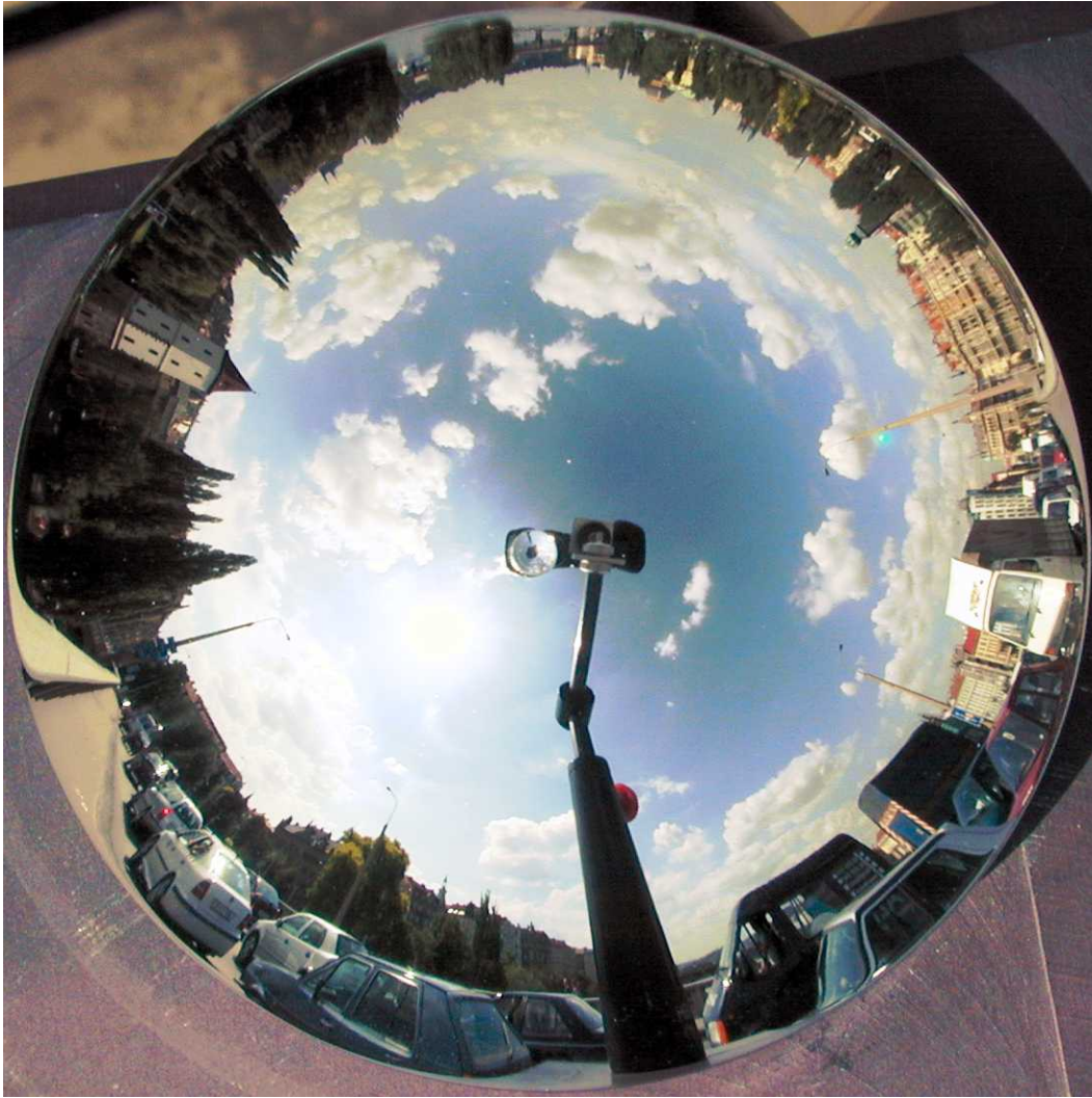
Fig. 1. An omnidirectional image obtained using a hyperbolic mirror and an ordinary perspective camera. Note the typical predominance of the sky in the image.
