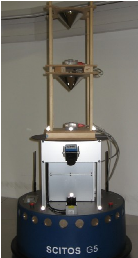
Fig. 14. DaX, the Scitos G5 mobile robot with two coaxial mounted conical mirrors and two firewire cameras.
