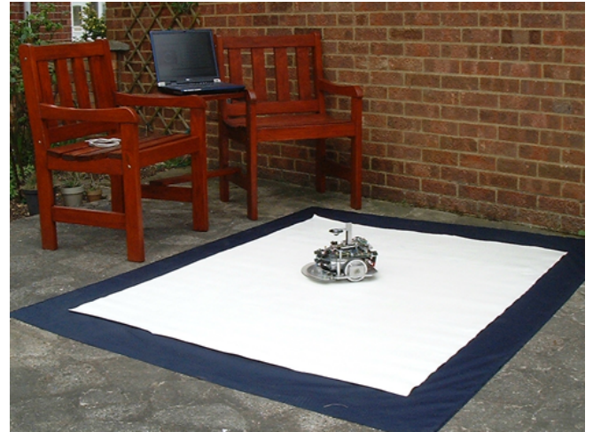
Figure 5: Test Arena. The area consists of a sheet of white vinyl approximately 1.5m by 1.25m. It is shown here resting on a darker sheet to improve the contrast of it's edge against the light coloured concrete.
