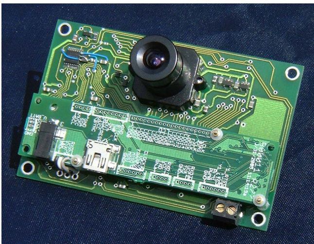
Figure 4: The new integrated vision module (based on the Kodak KAC-9618 image sensor). Overall Size: 83 x 54 x 30mm
