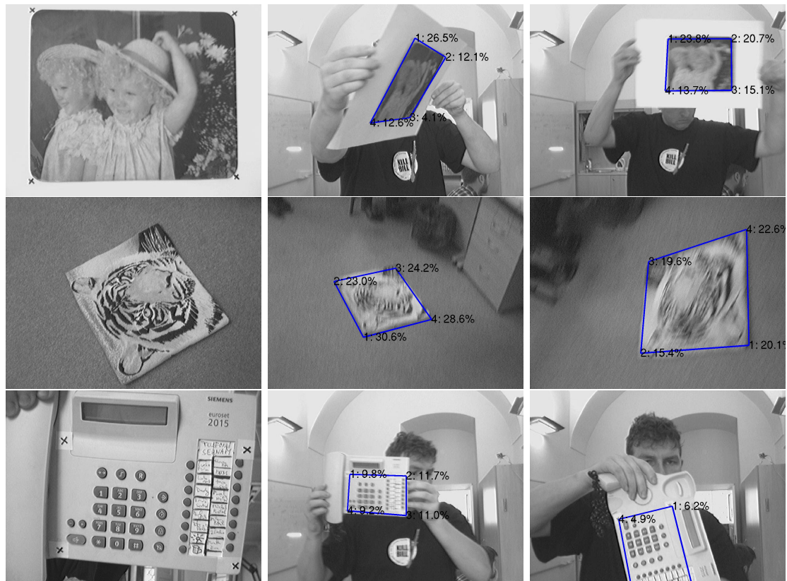
Figure 6.4: Ground truthed sequences: Left column shows images used for training. The middle and right columns demonstrate some successfully tracked frames with strong motion blur from the testing sequences. Blue rectangle delineates the object. Percentage values in corners are current corner speeds related to the current size of the object upper edge.
