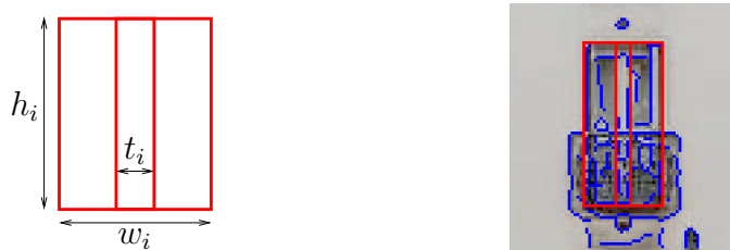
Fig. 2. Left: Window shape template is parametrized by its width w_i \in (0, 1) , height h_i \in (0, 1) , both relative to image height I_h , and the width of the central column t_i \in (0, 1) relative to the window width. Right: Shape template (red) is matched with image edges (blue).
