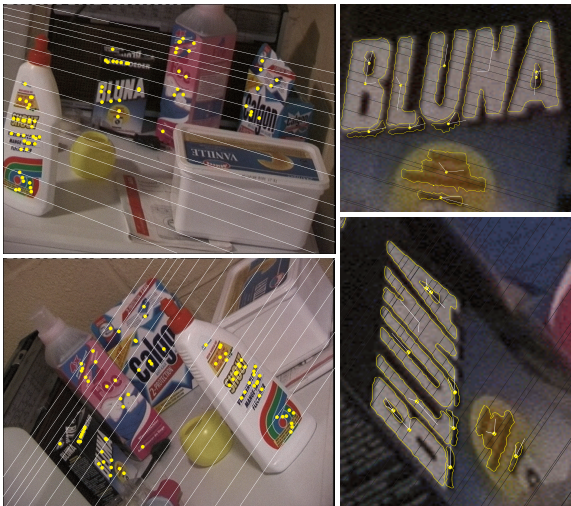
Figure 4: Epipolar geometry estimated on the 'Wash' image pair.
