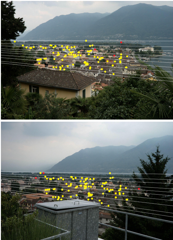
Figure 6: Epipolar geometry estimated on the 'Ascona' image pair.
