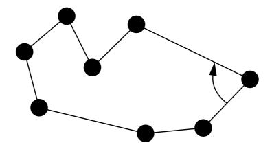
A sharp angle at a control point means a high curvature. We then use
