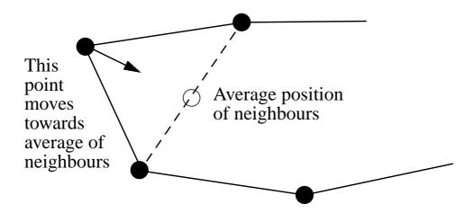
Easy to implement: to find the coords of the average of the neighbours, just average their *x* and *y* coords separately. Move the point by some fraction of the vector from its current position to the average position. (Usually calculate all the moves before actually doing any of them.)
