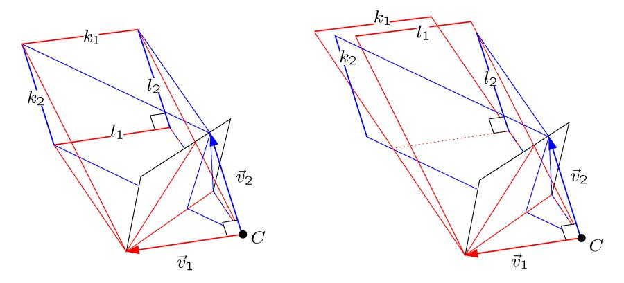
We will now show how to calibrate the camera by fining the matrix  $\omega = \mathbf{K}^{-\top}\mathbf{K}^{-1}$  from at least three vanishing points in general position.
