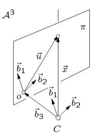
Miracle: The coordinates od the direction vector of a projection ray can be constructed by a adding "1" to image coordinates:
