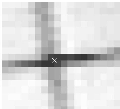
Figure 6: Detail of the calibration grid with manually detected control point (marked with 'x')
