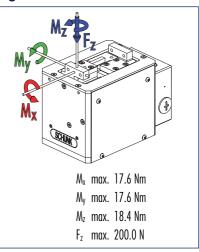
① Moments and forces apply per base jaw and may occur simultaneously. My may arise in addition to the moment generated by the gripping force itself. If the max. permitted finger weight is exceeded, it is imperative to throttle the air pressure so that the jaw movement occurs without any hitting or bouncing. Service life may be reduced.
