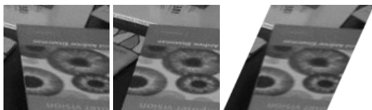
Figure 2: Left to right: Rectified sample of left image, rectified sample of right image, left sample transformed by an affine transformation to match right sample.
