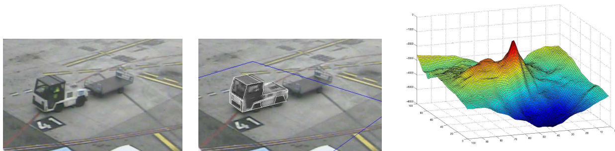
Figure 2: (Left) Frame of sequence S21 showing a transporter vehicle. (Centre) A 3D appearance model fitted to the vehicle, with the ground-plane (x,y) search area shown in blue. (Right) x,y -slice of the evaluation score surface in the (x, y, \theta) search space.
