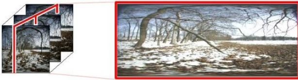
Figure 10: The whole IBR images is presented to the user in case of the linear motion. Additional scaling works on the columns only.
