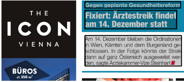
Figure 1: Text regions described in the source XML, visualized by rectangles. The text in the image on the left is not recognized as such, because it is part of the image itself, which depicts an advertisement.
