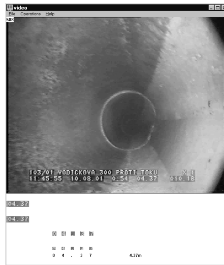
Fig. 5. Screen shot. Robot 2, 'satellite' camera on a string able to inspect lateral pipes, standard VHS showing the quality of input images and demonstrating processing.
