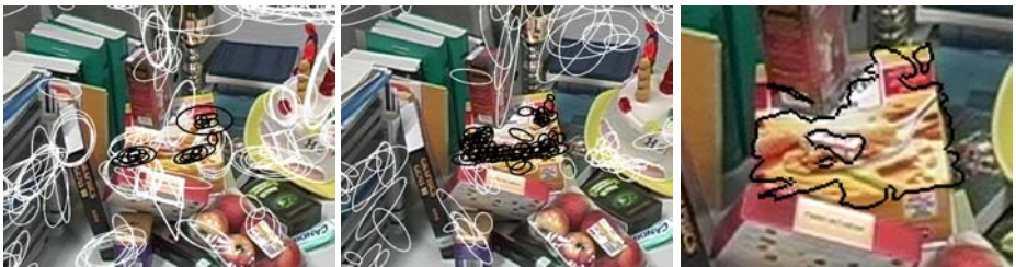
Fig. 4. Case-study. Left: 20 correct matches (dark) out of 330 after early expansion. Middle: 74/243 after the first main expansion. Right: contour of the final set of matches. Note the segmentation quality, in particular the detection of the occluding rubber
