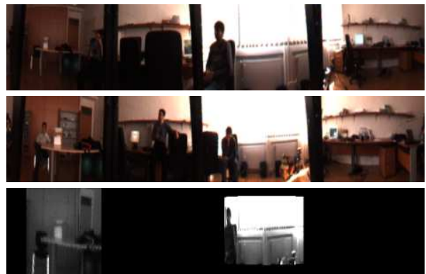
Figure 7. Top: one of the input images. Middle: an example of a query image. Note changes in the scene. Bottom: the closest X-slits image for the above query image. Note that only a small part of the scene could be rendered but it was sufficient to localize the robot. Only the intensity value of the pixels from the input set is used, thus the X-slits image is shown in gray scale.
