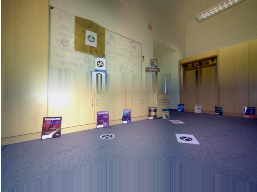
Figure 5: The resulting wide field of view image stitched from the six narrow field of view images shown in Figure 4. The middle and bottom parts of the image were not contained in any of the source images and were inpainted.
