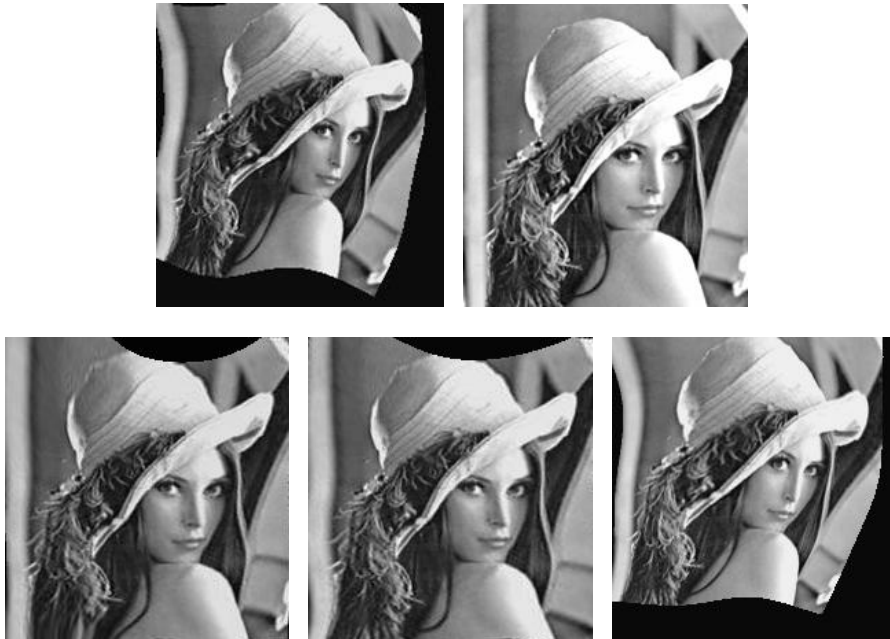
Fig. 2. From top to down, left to right: source image, target image, registered source image (by the standard method), registered source image (by our new method), registered target image (by our new method)
