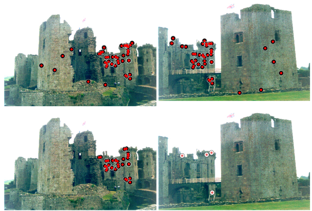
Figure 4. Image pair 19-22 in the Raglan scene. Points satisfying EG of this image pair (top row). Non-mismatch candidates identified before the multiview registration (bottom left). The four points used for translation registration (bottom right).
