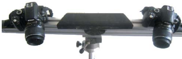
Figure 2. Kinect and two Nikon D60 SLR cameras rig.
