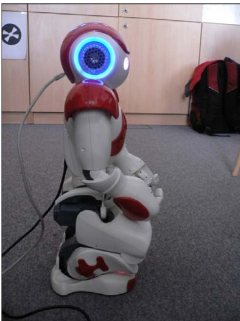
An example of a position in which the knee-motors will not overheat.
