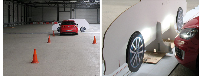
Fig. 12. Location of impact without intervention in VeHIL testing (left) and detailed view including laser measurement of target (right).
