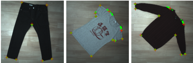
Fig. 8: Displacements of the vertices found by model matching (plotted in green) and the manually annotated landmarks (red). The displacements were computed for various configurations of garments and then they were projected to the canonical image.
