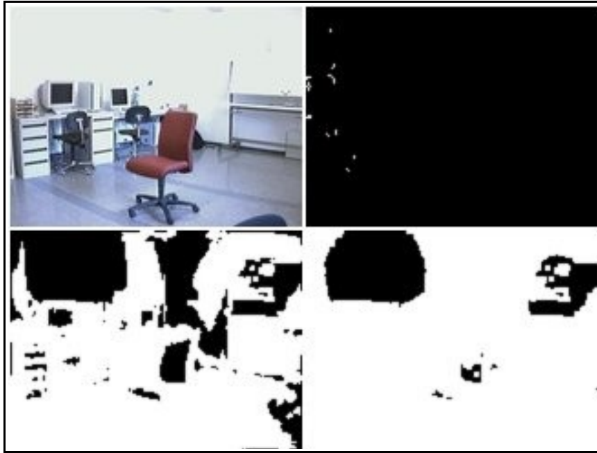
Figure 16. Frame number 203. The lights are turned on, and almost all the pixels are considered foreground, except the smooth areas.
