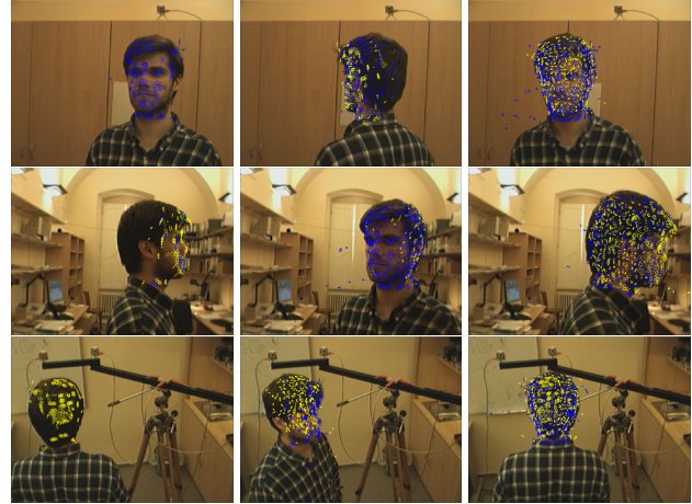
a) Multiview tracking; blue are visible, yellow invisible (occluded) projections
