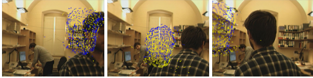
Monocular tracking results as projected to a camera which approximately orthogonal to the tracking one.
