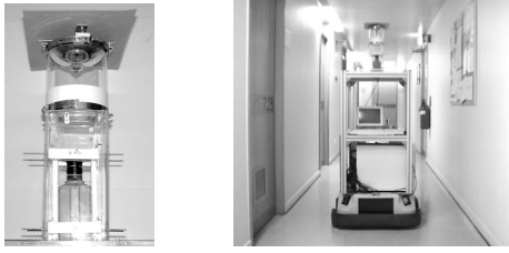
Figure 1: Left: the omnidirectional camera. Right: the camera mounted on the mobile robot.
