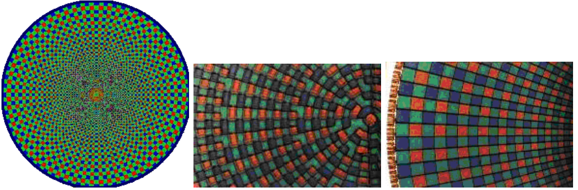
Figure 1: General view of the SVAVISCA Log Polar Sensor (left). Detailed views of the foveal (center) and retinal (right) regions.
