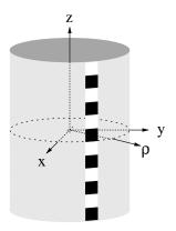
The mirror shape is given, when describing the problem by means of ray optics, in the form of a differential equation. Parameters to be designed are the desired *field of view* and the *cylinder radius*.
