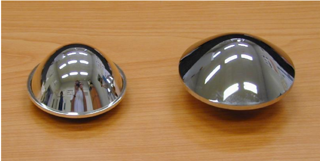
Figure 16: right: Hyperbolic mirror realized with chrome coating of a brass core; left: alternative technology based on aluminum coating of a glass core (shown here for an hyperbolic mirror).
