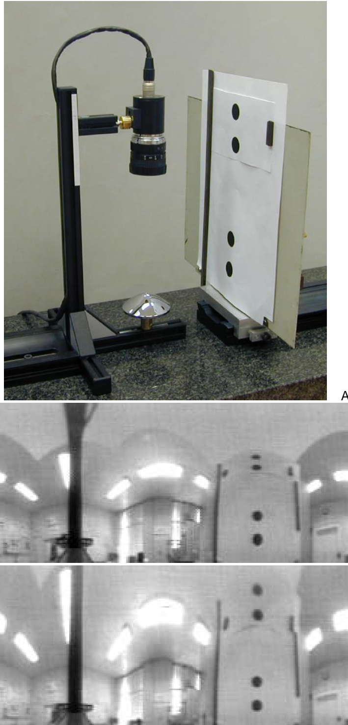
Figure 6: A) Set-up with a test pattern composed of black dots at the same distance but at different elevation. B) Image acquired with an hyperbolic mirror; C) Image acquired with the OMNIVIEWS mirror. The size of the dots are the same in C while in B they are different. In both cases the images are shown as they are acquired (i.e. no remapping and warping is required).
