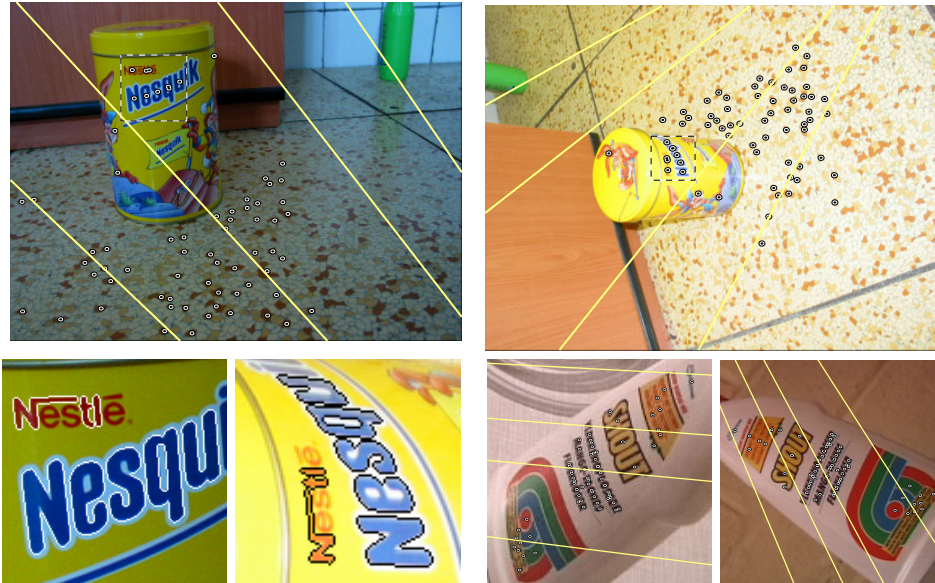
Figure 5: CYLINDRICAL BOX: Epipolar geometry (top) and matched regions (bottom left). Fully affine distortion, a non-planar object, textured surface and a strong specular reflection are present in the scene. SHOUT (bottom right), a scene with a change of illumination spectral power distribution.
