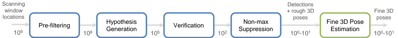
Fig. 2. Evaluation cascade of the proposed method. Note the typical numbers of detection candidates advancing through individual stages (for a template size 108 \times 108 px, a VGA input image and a scale space with four larger and four smaller scales with a scaling factor 1.2). A detection candidate is a triplet consisting of a template identifier (object and its orientation), a sliding window scale and a sliding window location.
