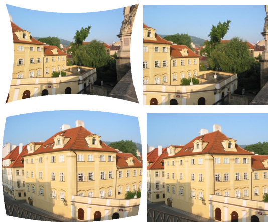
Figure 1. Real data. (Left) Input images with different radial distortions for left (Top) and right camera (Bottom). (Right) Corrected images.
