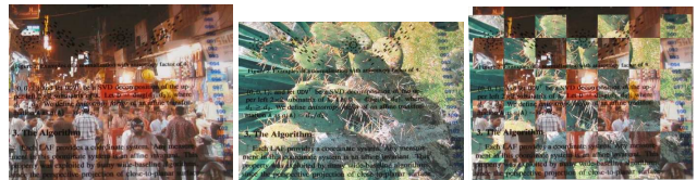
Figure 7. Two photographs of a text on a transparent foil, each time on a different background, and their superposition after successful registration.
