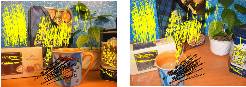
Figure 7.5.: Motion segmentation. The motion of the background and the foreground (the mug) are denoted by light and black lines respectively.
