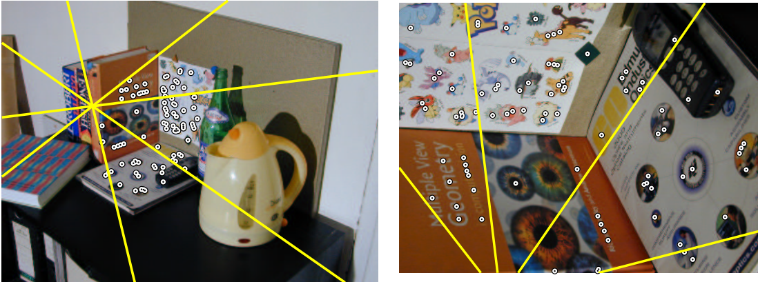
Figure 5.5.: Epipolar lines and 84 detected correspondences (markers) superimposed over the ‘Bookshelf’ pair.
