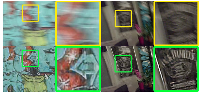
Figure 1. Heavily blurred images captured with a fast moving camera (top). Images deblurred by DeepGyro CNN (bottom).
