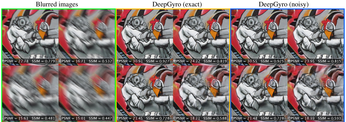
Figure 6. DeepGyro performance for increasing levels of blur. Blurred images (green). Results obtained when passing the exact blur \epsilon = [0, 0] as input (orange), and when the blur vector has an error \epsilon = [5, 3] pixels (blue). Testing with blur sizes: 10, 40, 60, 80 pixels.
