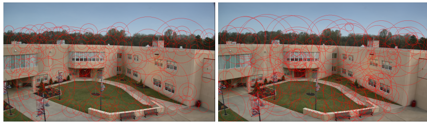
Figure 4.8: Two approaches to sampling of patches. Left: using a probability map, right: using multiscale Hessian detector with scale-wise nonmaxima suppression. Both variants contain 186 patches. Patch centers and scales marked on single AMOS Views image.
