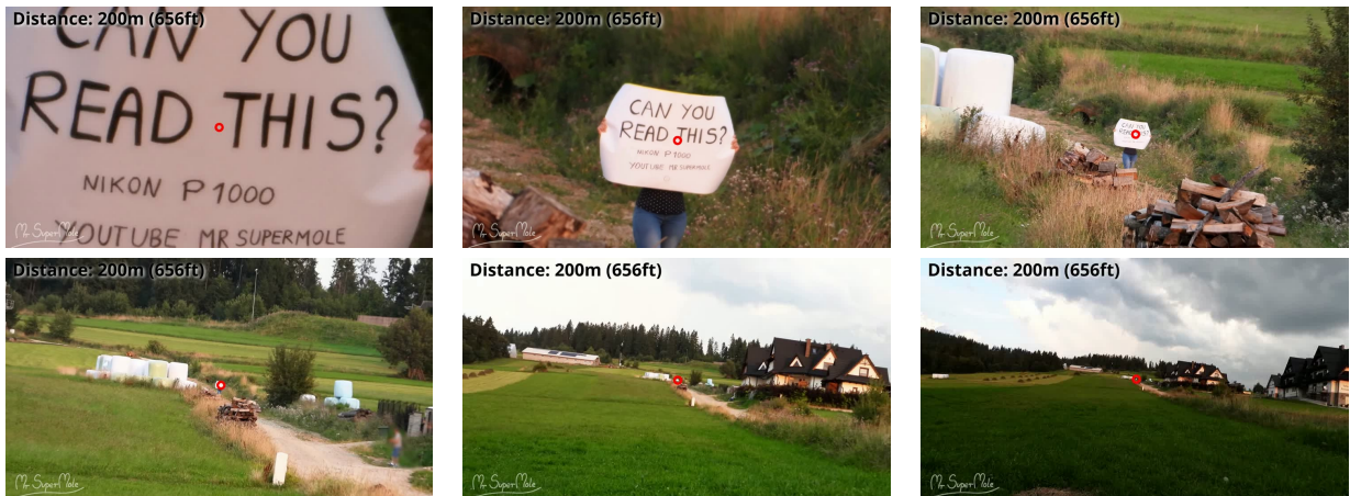
Figure 25: MFTIQ failure case. Example of a video with zooming out. Every 100th frame shown. Even with flow correctly chained (red circle) it is impossible to estimate the occlusions and uncertainties directly between the first and the last frame. Video source: https://www.youtube.com/watch?v=r1bIXAV9Cnc
