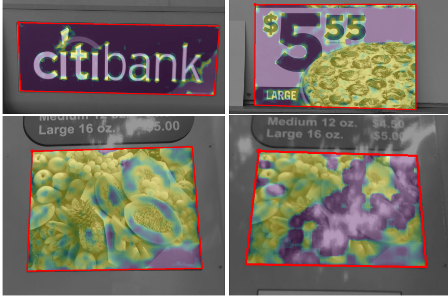
Figure 5: High weights of optic flow ( yellow ) appear mainly on corners and well-textured areas. Bottom : the POT-210 target with the highest average flow weights ( left ); weight values drop ( purple ) when “occluded” by a reflection ( right ). Best viewed in color.
