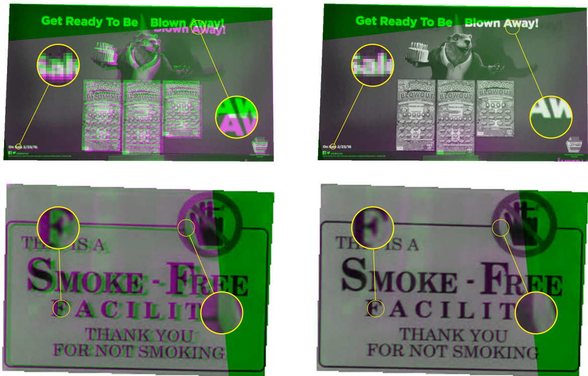
Figure 7: Precise re-annotation examples. Original ground truth annotation ( left ), improved ground truth annotation ( right ). The grayscale template in green channel, the GT-warped current frame in red and blue channels. Imprecise annotation causes green and magenta shadows, while precisely aligned images produce a grayscale result. The green bands on top and on right side respectively are caused by a partial occlusion on current frame. The alignment error of the original GT evaluated on the improved ground truth is 15.8px ( top ) and 7.2px ( bottom ).
