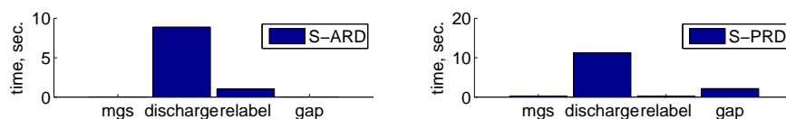
Figure 23 Workload distribution, for size 1000 \times 1000 , connectivity 8, 4 regions, strength 150. msg – passing the messages (updating flow and labels on the boundary), discharge – work done by the core solver (BK for S-ARD and HPR for S-PRD), relabel – the region-relabel operation, gap – the global gap heuristic.
