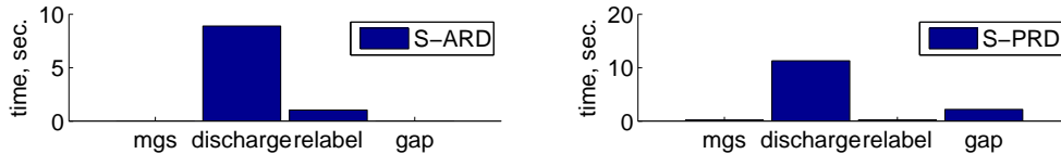
Figure 10: Workload distribution, for size 1000 \times 1000 , connectivity 8, 4 regions, strength 150. mgs – passing the messages (updating flow and labels on the boundary), discharge – work done by the core solver (BK for S-ARD and HPR for S-PRD), relabel – the region-relabel operation, gap – the global gap heuristic.
