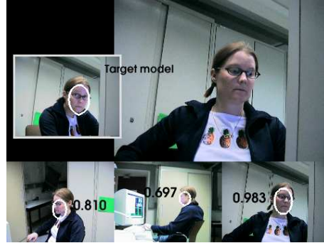
Fig. 3. The best view selection according to the Bhattacharyya coefficients of the individual trackers is shown. The small images on the bottom show the current tracking results of the individual camera views as white ellipses and the corresponding Bhattacharyya coefficients. In the top row the best target model and the output of the virtual editor are displayed.
