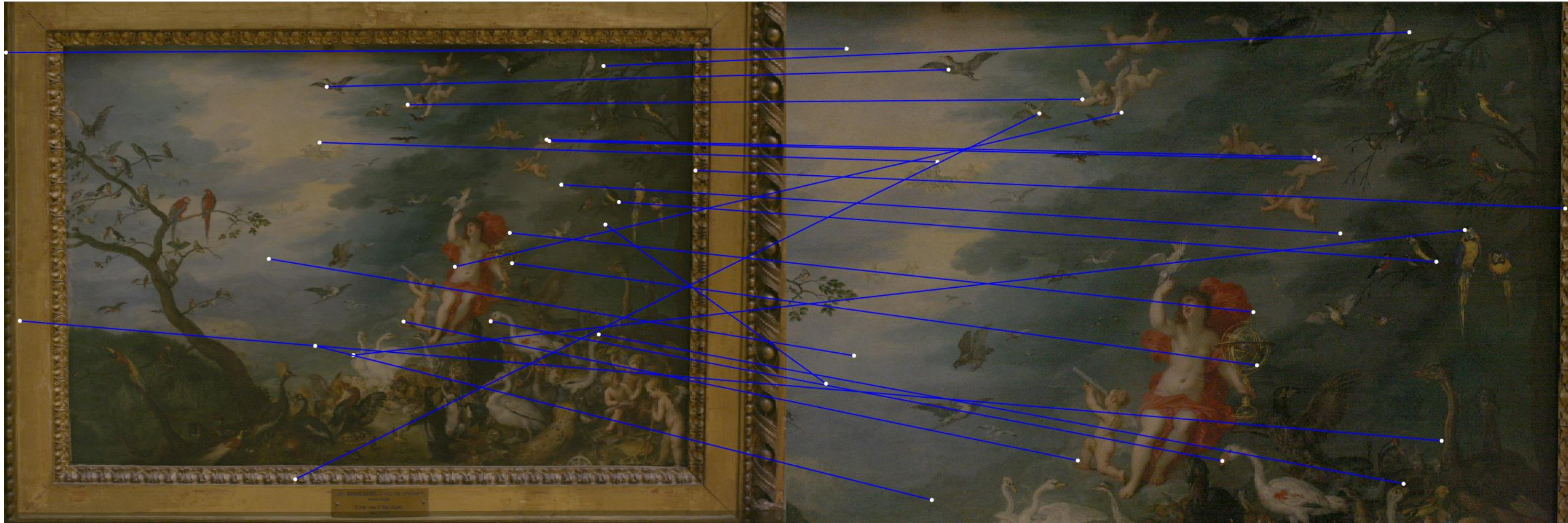
Point correspondences detected in an image pair.
