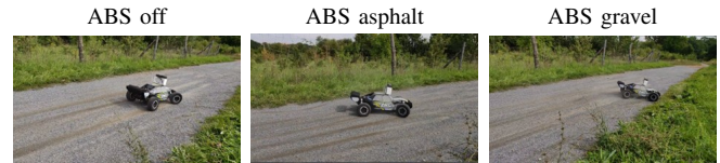
Fig. 10. Subscale vehicle ride tests. Photos capture the platform after performing the collision avoidance maneuver on gravel. The operator initiates full braking immediately followed by the full right steer command.
